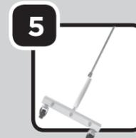
Direct water supply into quick connect (a) on broom for 30 seconds to flush out loosened particles.
