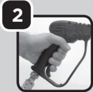
Depress the trigger on the gun to begin spraying. Release trigger to stop spraying.
