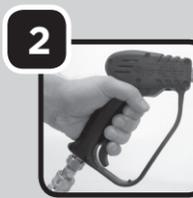
Pull trigger on gun handle to relieve any water pressure.
