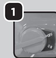
Shut off pressure washer and turn off the water supply.
