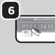
Reassemble the nozzles to the water broom using teflon tape to prevent leaks.
