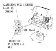
Use 12V and more than 45A·H battery, connect its positive lead to start relay terminal while connect its negative lead to engine mounting screw, base screw or other grounding point with the engine. (See Fig. 2)
